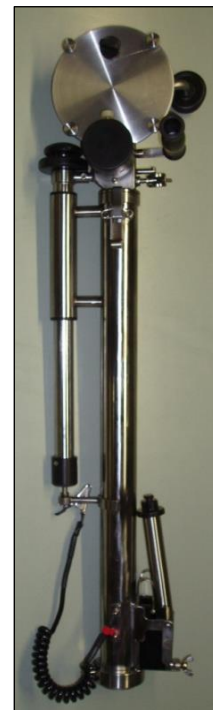
Winder MK 7, with Depth Counter & MMC type coupling
