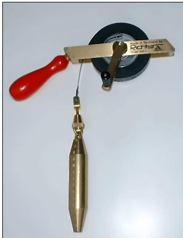
20 m tape on frame with 0.7kg weight
