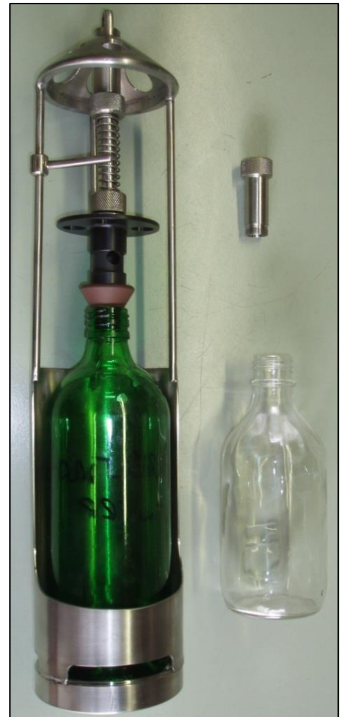
ALSB-V 1002, 1-litre & 500 ml bottles and showing short bottle adaptor
