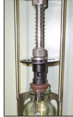
Inlet valve set to maximum opening (for viscous oils)
