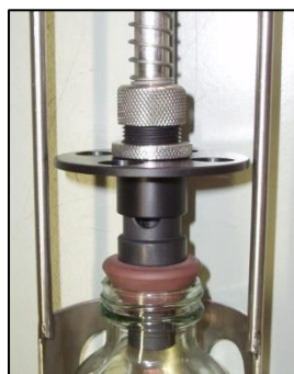
All-level Sampling: Inlet valve set to minimum opening (for light products)
